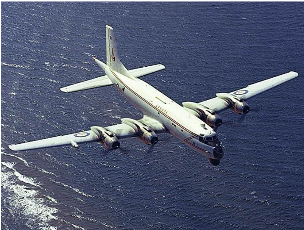
Mark 2 Argus 10731 on maritime patrol with the high intensity searchlight (70 million candle power) visible on the right wing.
