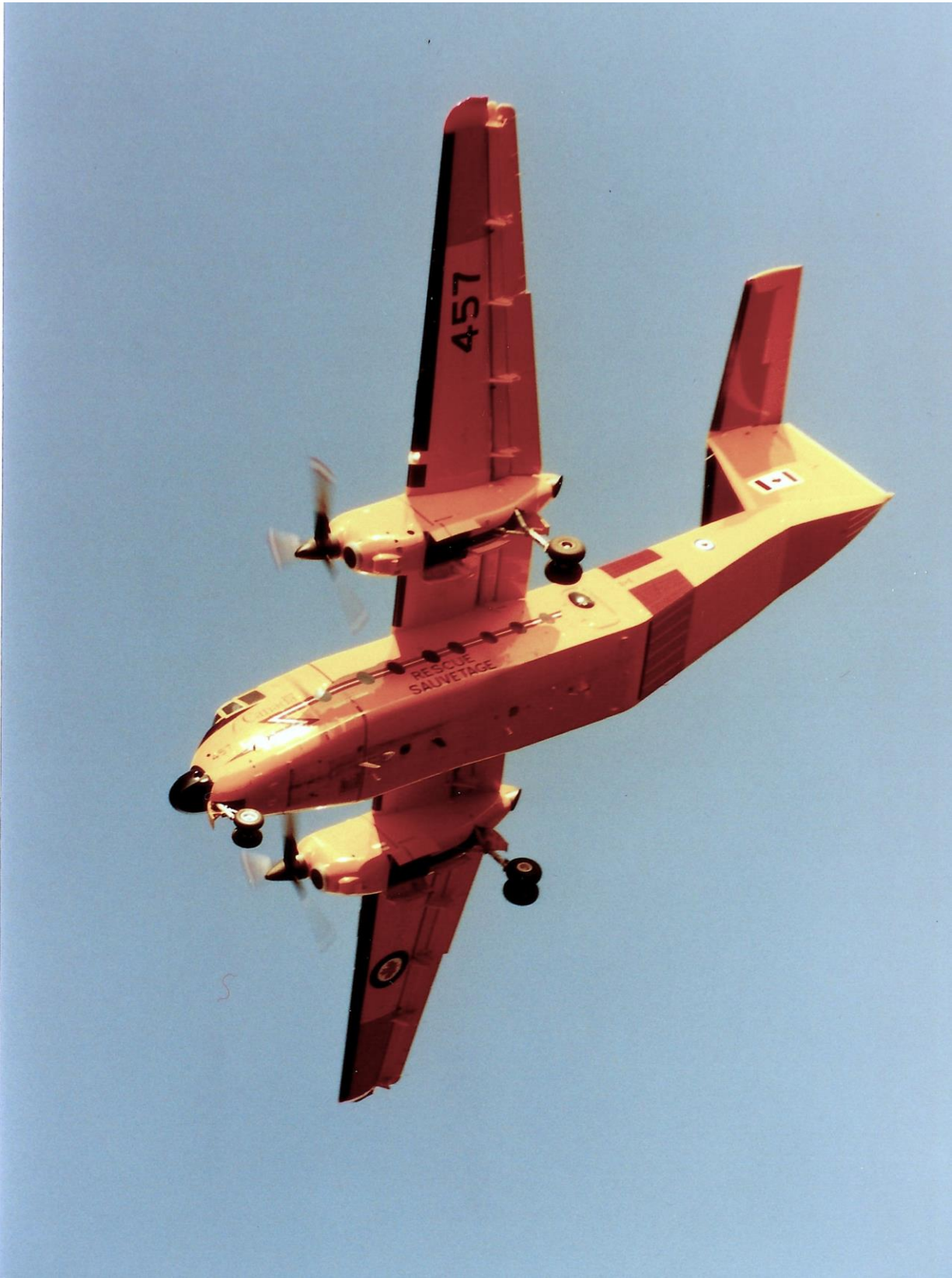
Dramatic shot of 115457 on approach for a STOL landing while in service with 442 Squadron, Comox, BC. As a STOL aircraft, it could land in 850 feet, reverse thrust on the propellers to back up for every available inch of runway, and then take off in 2,300 feet.
