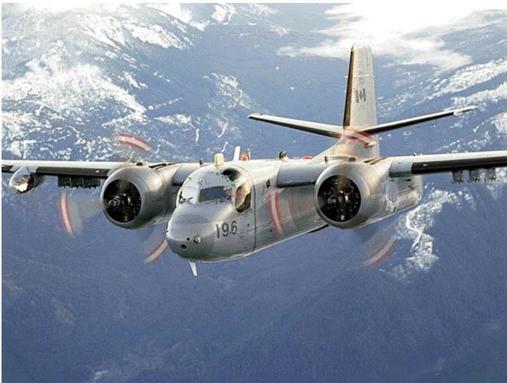
Tracker 12196. The Tracker is equipped with a 70 million candlepower searchlight for the identification of surface contacts at night and wing pylons to carry CRV-7 rockets.
