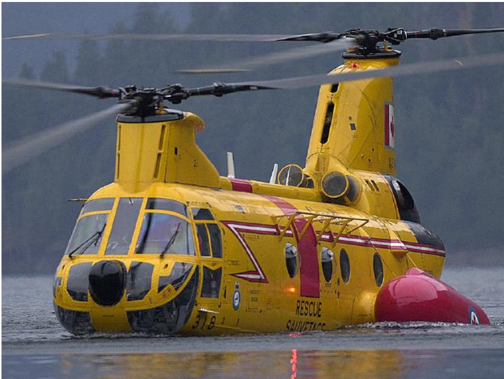
CH-113 Labrador 11318 showing off the watertight hull for marine landings. Note the FOD screens on the engine intakes.
