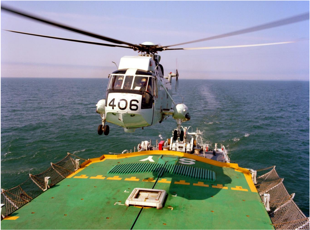
Sea King 12406 prepares to land on the deck of HMCS Saguenay. The Helicopter Destroyers (DDH) employed the “Bear Trap” Helicopter Haul-Down System...the square device on the flight deck (the Bear Trap), and the steel grid arrangement between the Bear Trap and the call letters of the ship “SY”. The Bear Trap was also used to move the Sea King into and out of the hangar.
