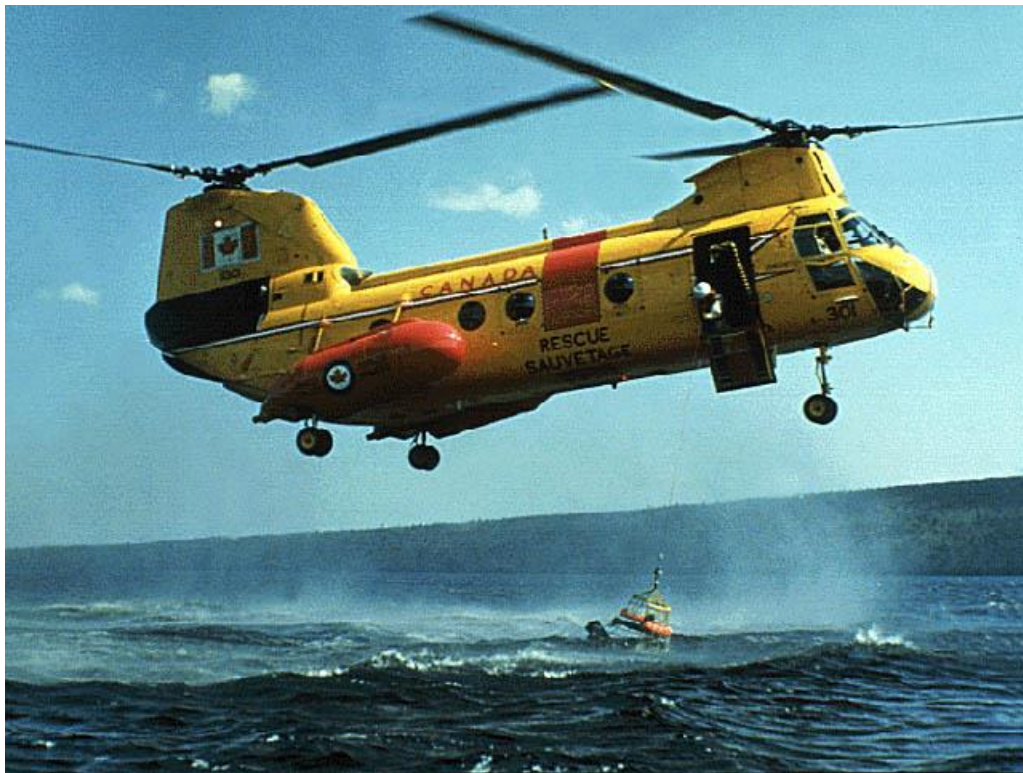
CH-113 Labrador 11301 plucking a person from the water using a “Billy Pugh” net on the rescue hoist. This is an early version of the Labrador. Note the rescue hoist is the “original” style contained inside the rescue door; later it was mounted outside and above the door. Also, there is no nose radar radome.
