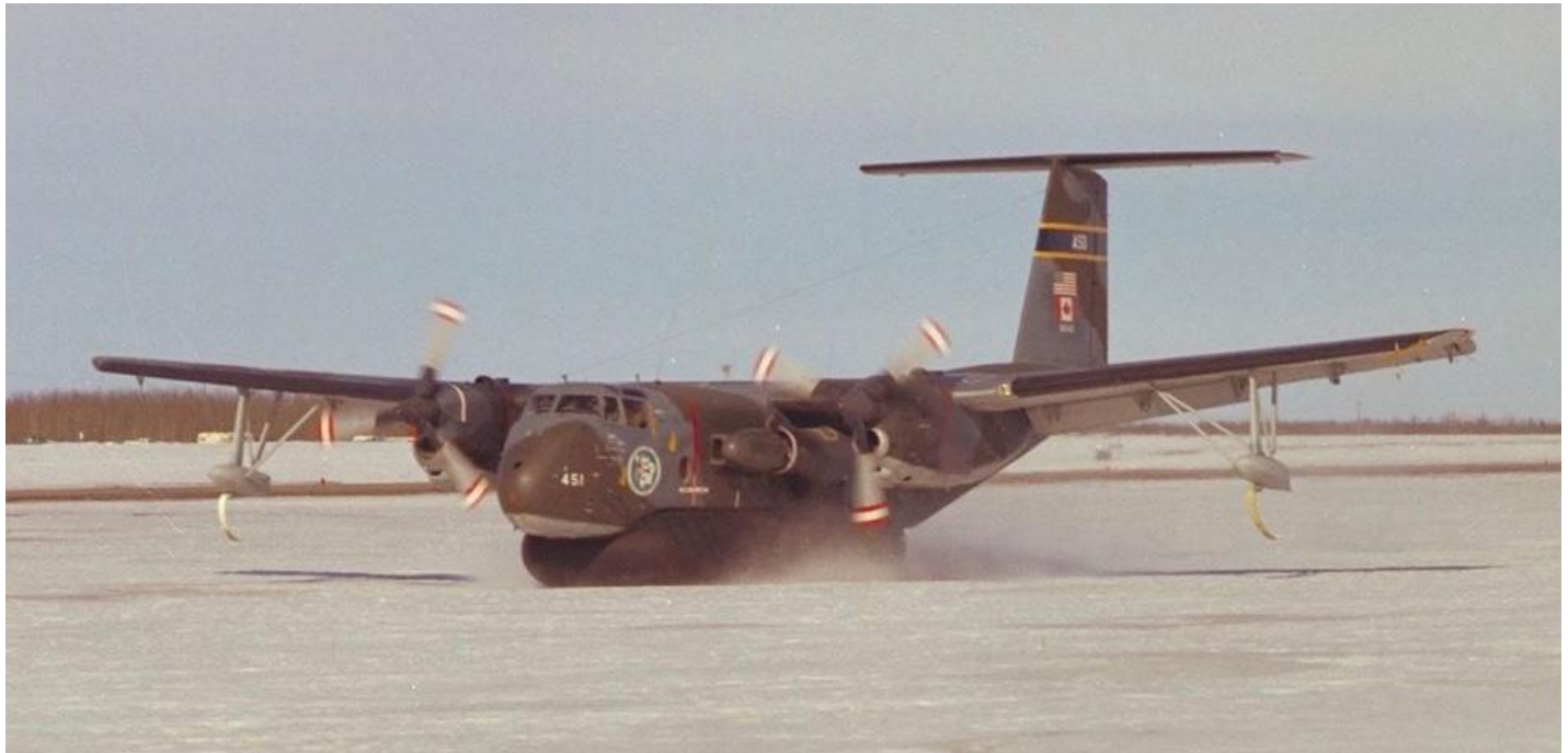
115451 during air cushion trials with Bell-Textron. It utilized two jet engine driven compressors for the belly air bag and wing outriggers for stability.
