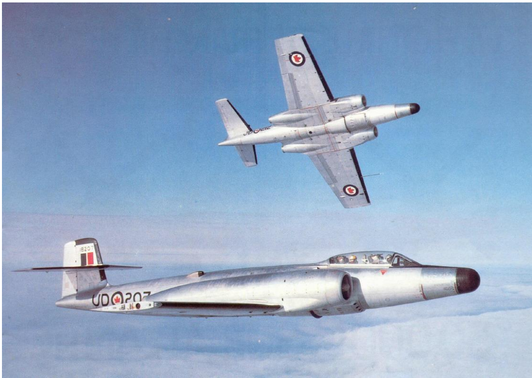
A pair of 419 Squadron Mark 4A Canucks (18207 and 18212). The plan view of 18212 shows the Mark 4 wingtips without the extensions of the Mark 5 aircraft. Also note the extended nose as compared to the bullet-shaped nose of a Mark 3. Note the one-piece canopy of Marks 4 and 5.
