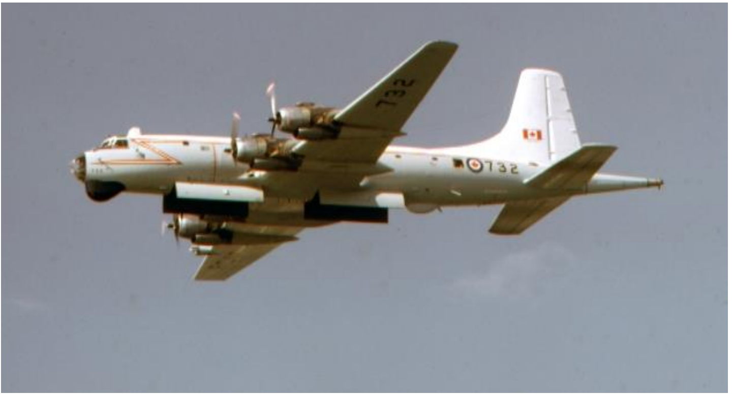
Mark II Argus 20732 with it's fore and aft bomb bay doors open. Aft of the bomb bays are chutes to drop sonobuoys into the ocean. A sonobuoy is like a microphone which can hear submarine engine and propeller noises. (29 Aug 1968, Canadian International Air Show, Toronto)
