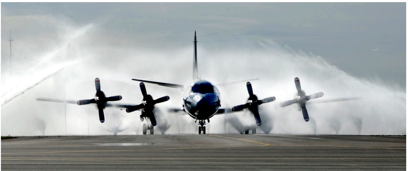
An Aurora in the Birdbath. While flying over the ocean, tiny particles of salt adhere to the surface of the aircraft and must be removed before they corrode the metal. The fresh water of the Birdbath rinses it clean.
