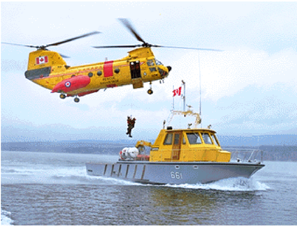
CH-113 Labrador using the rescue hoist during a live hoist exercise. This updated Labrador has the improved high-speed rescue hoist mounted over the side door and a nose-mounted weather radar.
