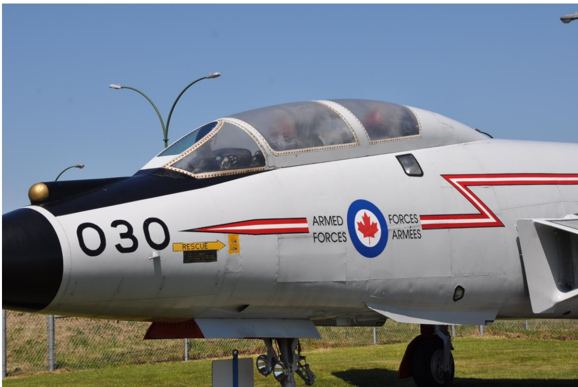
CF-101B, 101030. Note the infra-red seeker head on top of the nose, and the anti-corrosion, light grey paint.
