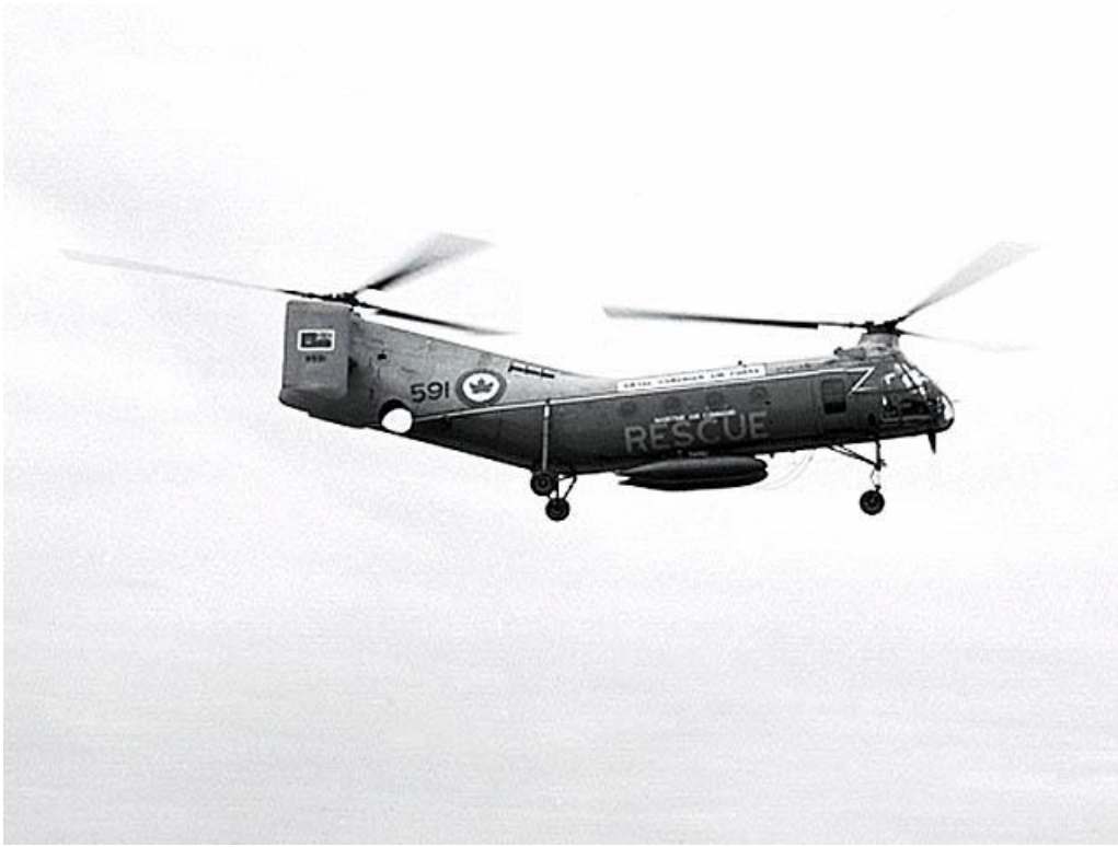
Vertol H-44A 9591 shown with two auxiliary 165 US gallon (625 litre) fuel tanks. Either one or two could be carried and the tanks could be jettisoned by the pilot or a crew member. (RCAF Photo)
