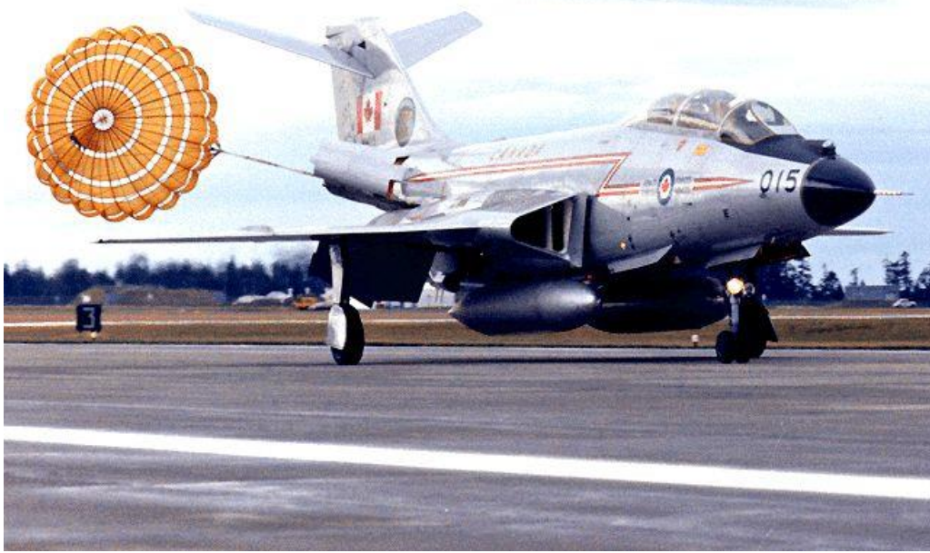
CF-101B, 101015, on active duty with 409 Squadron hangs on the drogue 'chute as it completes a landing roll out at CFB Comox in 1975. Of note, are the twin, large diameter, 450 US gallon (375 Imp Gal, 1705 Litre) drop tanks.
