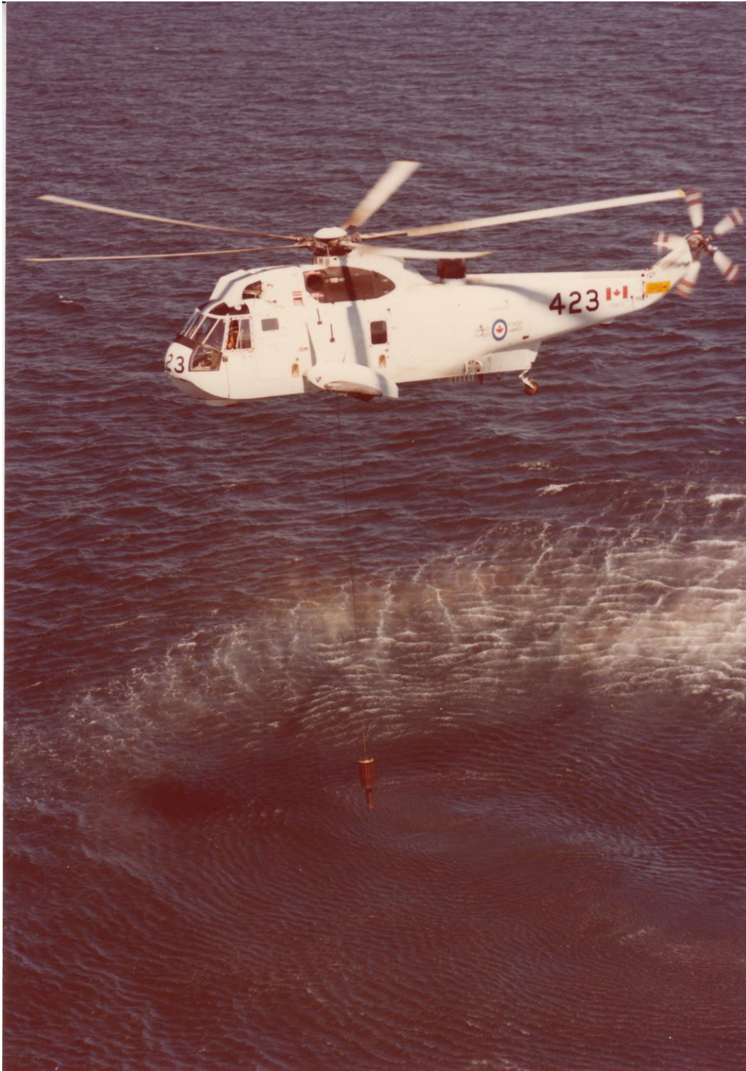
Sea King 12423 in its normal working position, in a hover, 50 feet above the ocean and lowering its dipping Sonar ball into the ocean...known as "in the dip". The Sonar ball detects submarine noise (from its engines, etc.) to enable the Sea King crew to locate the submarine. The Sea King is sporting the second paint scheme, a light greenish-blue.
