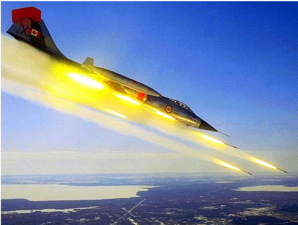
Canadair CF-104, 104704, is from the Aerospace Engineering Test Establishment (AETE) at Cold Lake and is firing Canadian-built CRV-7 rockets on the Primrose Lake Evaluation Range. The maximum rocket load of the CF-104 was 76 rockets.
