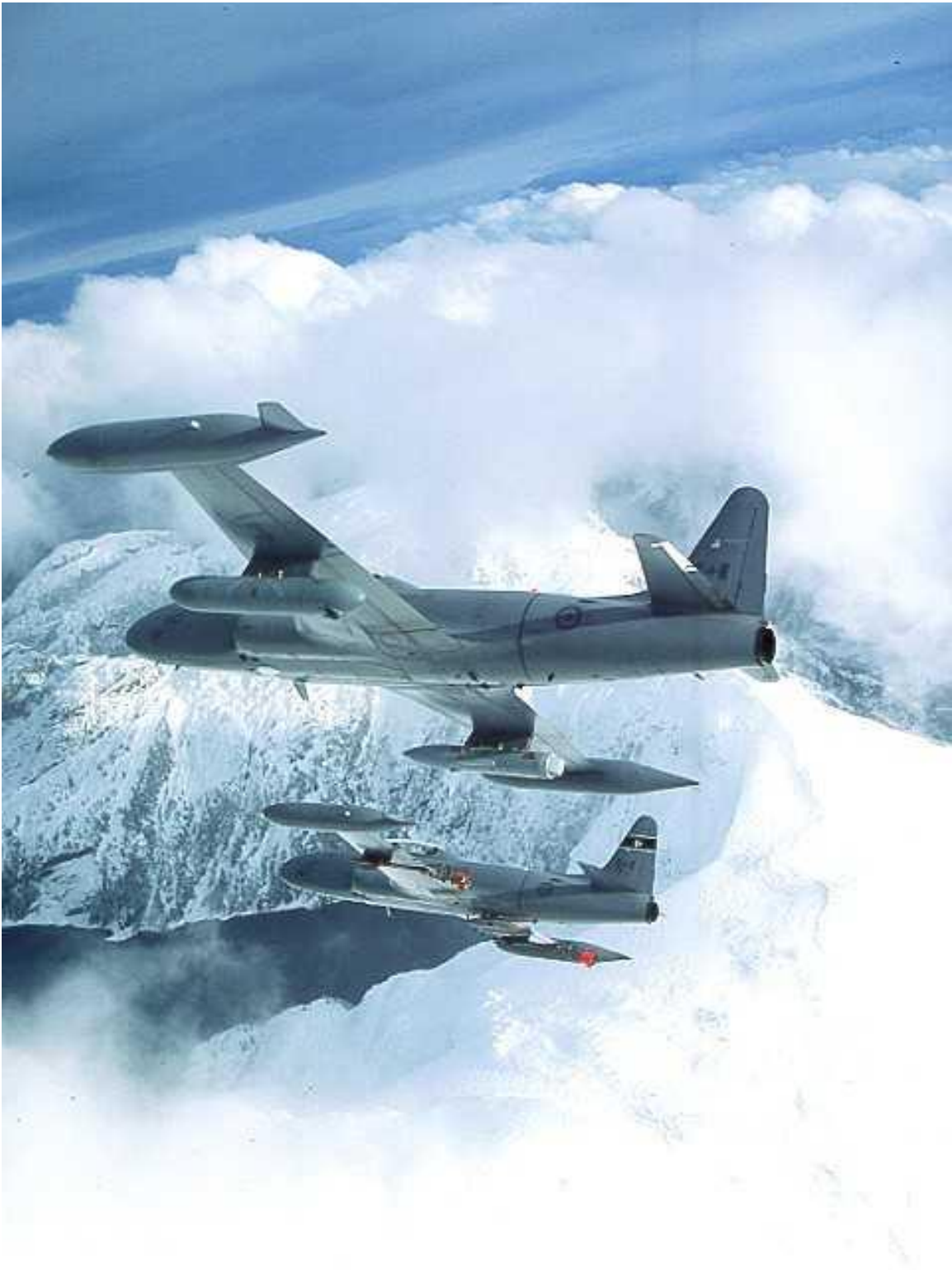
Two Electronic Warfare Silver Stars display some of the equipment that they carry on the under wing hard points. The lead T-Bird carries the missed-distance indicator under each wing which was used for assisting ships in surface-to-air gunnery while the second aircraft carries an ALQ-503 Electronic Warfare jamming pod under the right wing and an ALE-503 chaff dispenser under the left wing.
