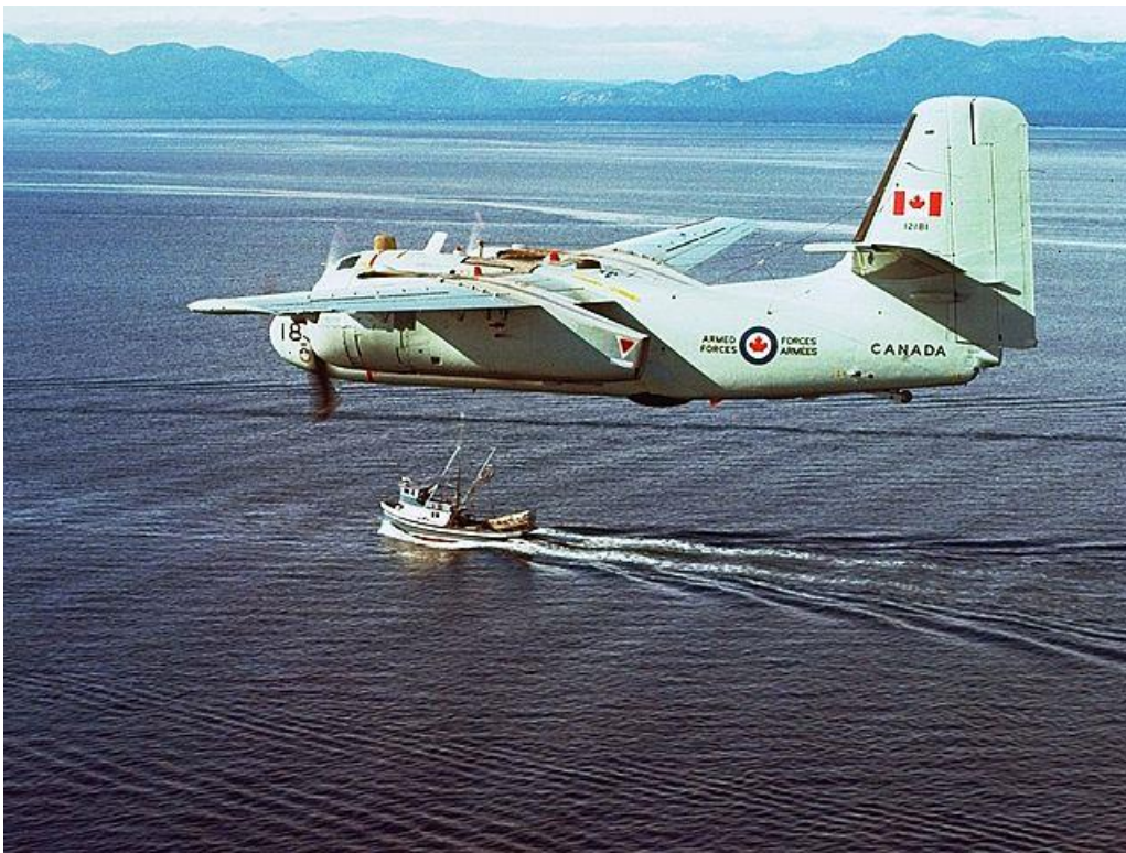
Tracker 12181 on fisheries patrol in the overall light blue paint scheme. Note the black radome of the search radar in the retracted position.
