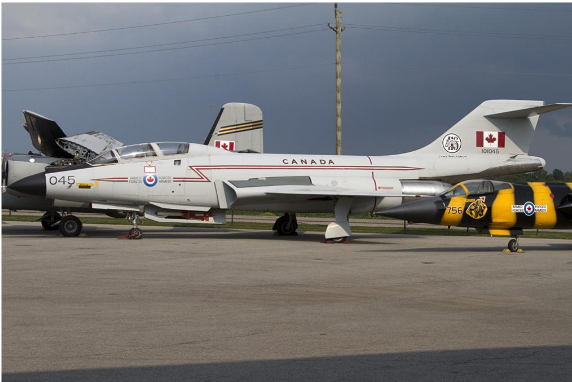
CF-101B, 101045, in 416 Squadron markings. Note the large size of the Voodoo as compared to the CF-104 Starfighter in tiger strip scheme beside it (104756, 439 Squadron). Also note the rotary weapons bay containing a Falcon missile, in the recessed position, just aft of the nose wheel of the Voodoo.
