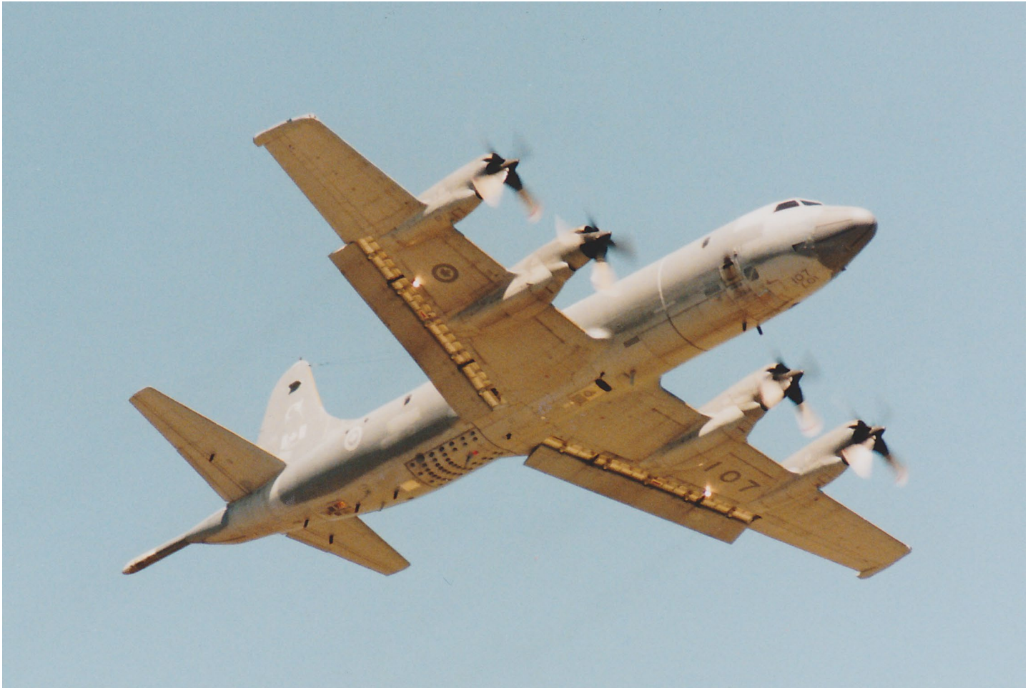
140107 when with 415 Squadron in Summerside, P.E.I., showing the belly of the beast. The flaps are down and on the fuselage aft of the wings are chutes to drop sonobuoys into the ocean. A sonobuoy is like a microphone which can hear submarine engine and propeller noises.
