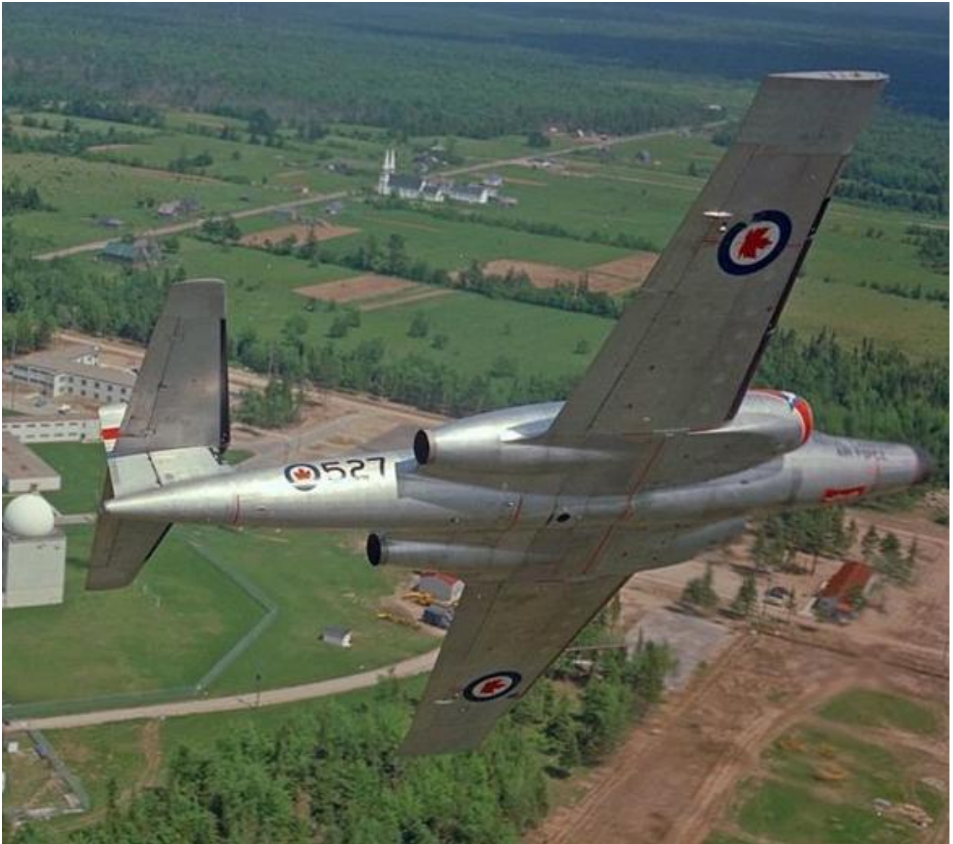
Mark 5 Canuck 18527 of 425 Squadron. This shot highlights the wingtip extensions added to the Mark 5. Also note the gun pack has been removed. (CF Photo)
