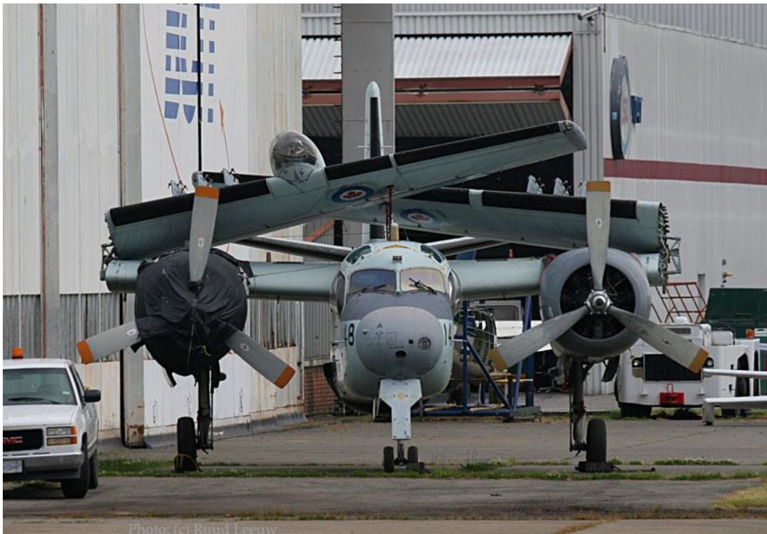
Tracker 12148 with wings folded to allow it to fit in the Bonaventure's hangar. Also, the Canadian Tracker was built 18 inches shorter than its American counterparts.
