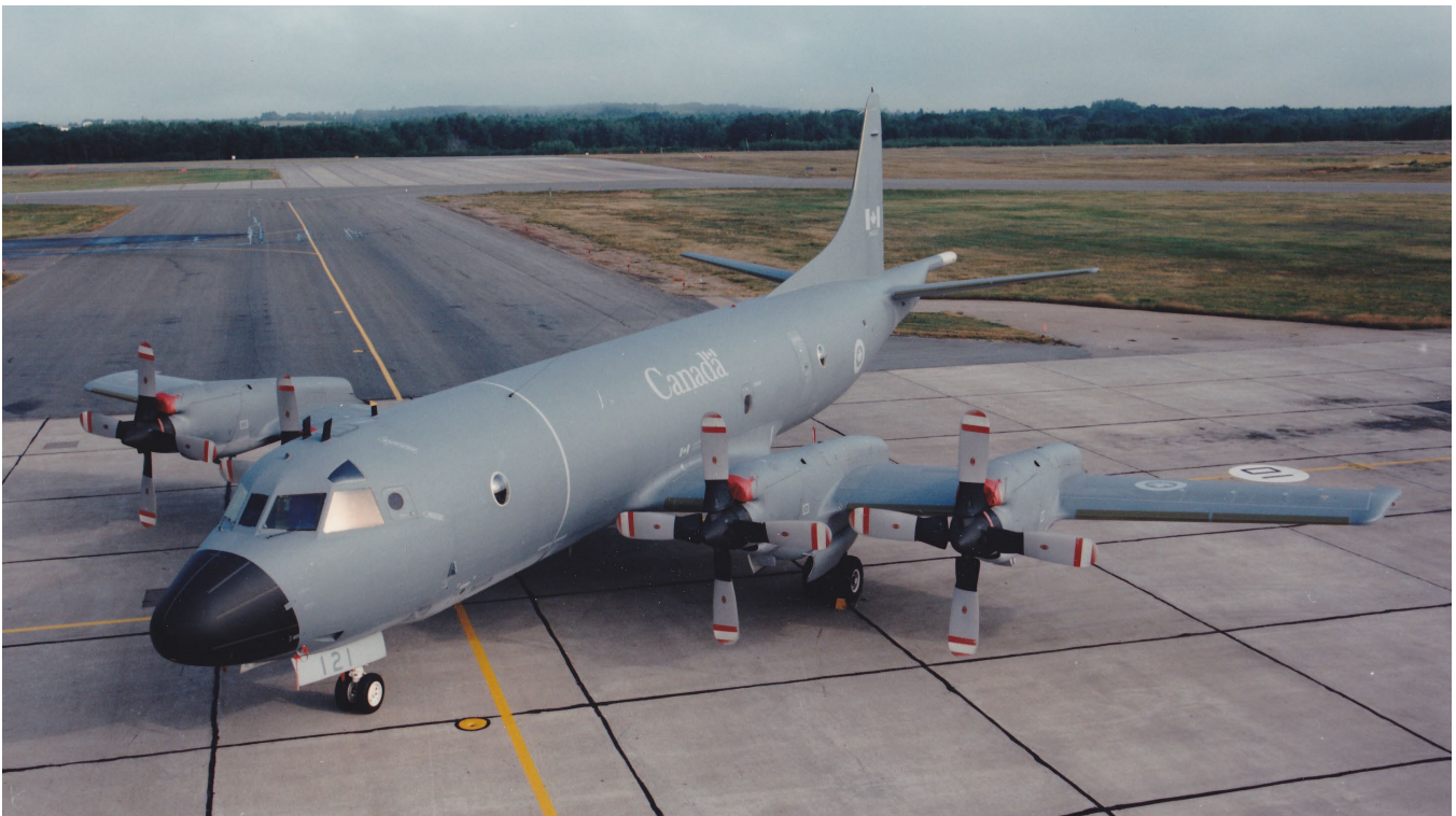
140121 Arcturus in Greenwood, Nova Scotia. Three sister aircraft of the CP-140 Aurora, the CP-140A Arcturus, were used to augment the Aurora fleet in monitoring Canada's Maritime Approaches and the Arctic. The Arcturus shared the same airframe as the Aurora, but was not equipped for anti-submarine warfare (ASW). Because it lacked the Aurora's heavy ASW electronics, the Arcturus was a lighter and more fuel-efficient aircraft.
