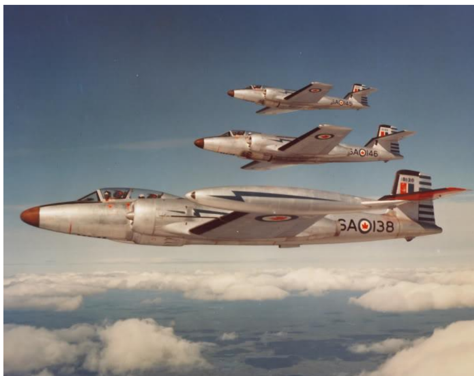
A flight of 445 Sqn, Mark 3 Canucks, 18138 has tip tanks whereas the other two (18146 and 18145) do not. The black smoke stains at the muzzle end and the aft end of the gun pack indicates they have just finished a training mission in the weapons range. Note the two-piece canopy of Marks 1, 2 and 3. (RCAF photo)
