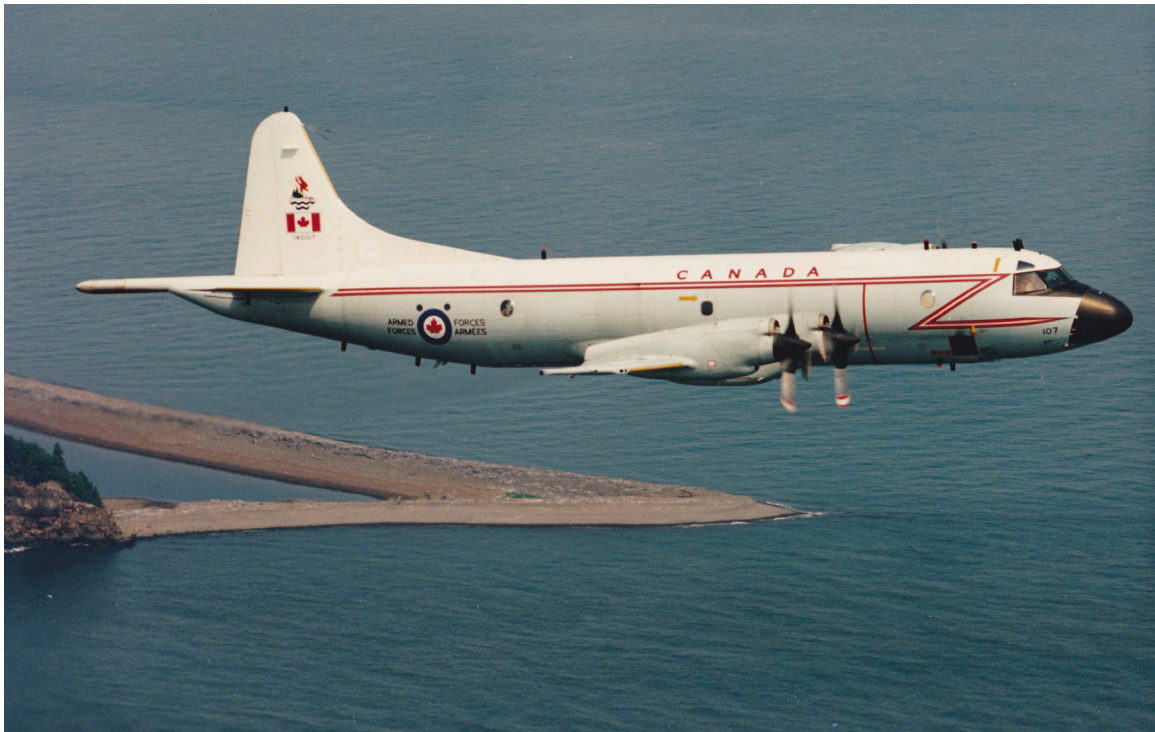
140107, a 405 Squadron Aurora from Greenwood, Nova Scotia, displaying the original paint scheme. Protruding from the tail is the MAD Boom, a Magnetic Anomaly Detector which detects the magnetic field surrounding a steel submarine.
