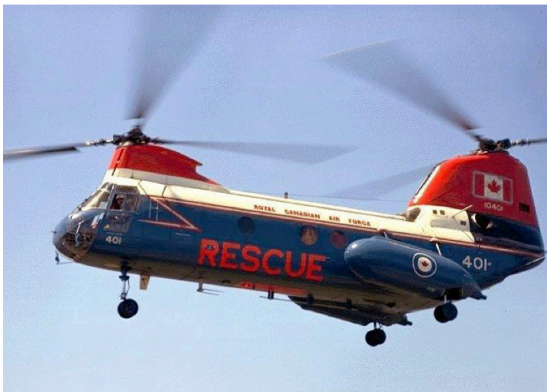
CH-113 Labrador 10401 shown in the original Search and Rescue colours. Note the larger sponsons on the Labrador.
