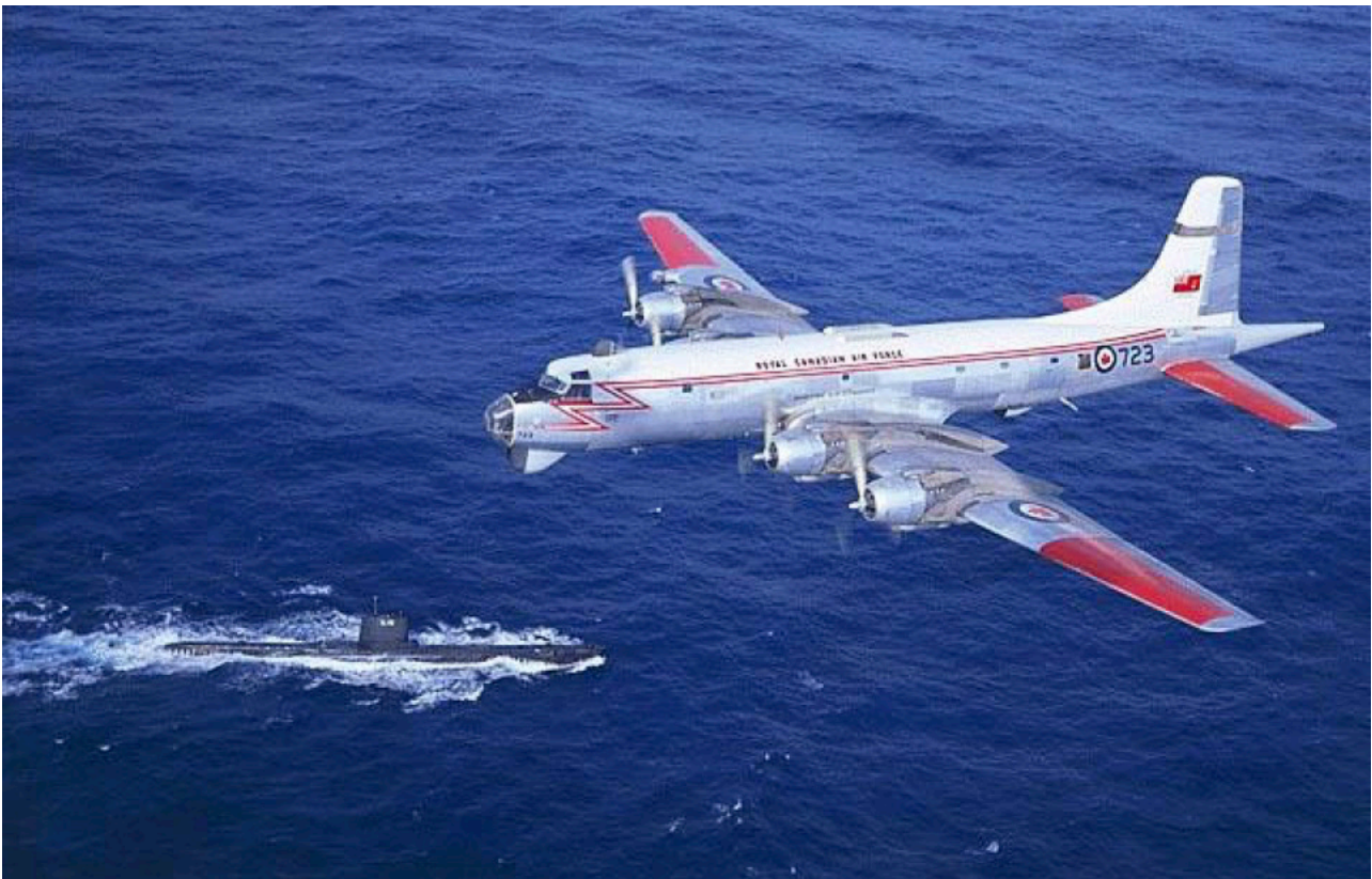
A Mark II Argus (20723) on maritime patrol visually identifies a Canadian Oberon-class diesel electric submarine. Note the smaller nose radome of the Mark II.
