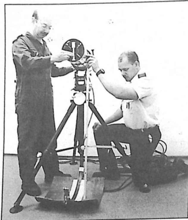
MCpl Edmundson and Cpl Brown preparing the X-ray machine for testing of an aircraft part.
