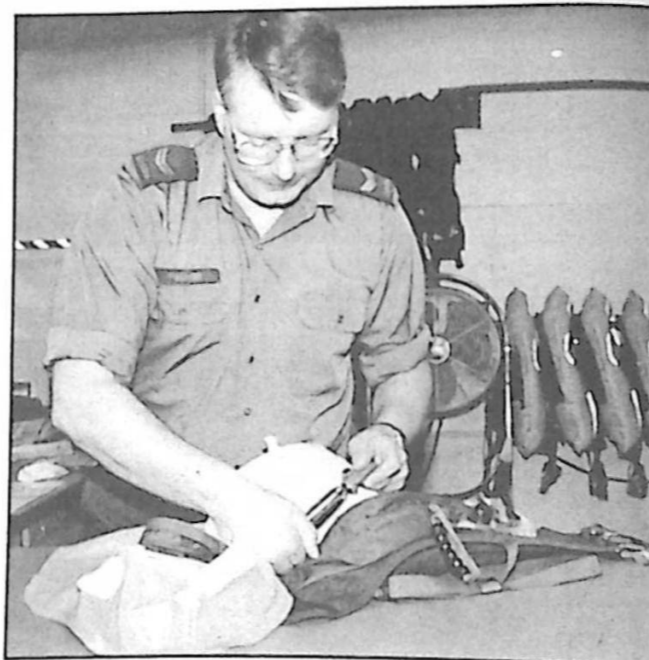
Cpl Palmer installing a carbon dioxide cartridge into a life vest. The CO 2 cartridge will instantly inflate the vest when activated.
