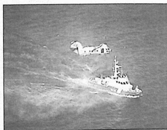
A Canadian military Labrador helicopter from 442 Transport and Rescue Squadron in Comox practices a boat hoist with the Canadian Coast Guard vessel Point Race near Cape Mudge on Quadra Island, B.C. on 8 July. The squadron uses this procedure to rescue injured people from fishing vessels, cruise ships and a variety of other vessels. In 1999, 442 Squadron crews carried out 246 air searches in the busiest search and rescue (SAR) zone in Canada.
