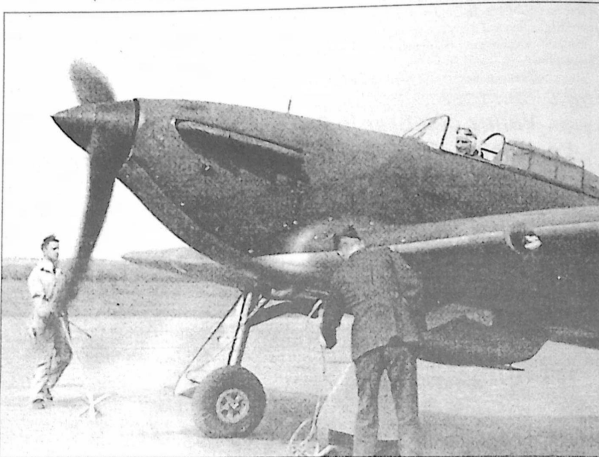
S/L E.A. McNab (now Group Capt McNab, O.B.E., D.F.C.) about to take off in one of No.1 Squadron's Hurricanes from Ottawa to St. Hubert. Top speed of this aircraft was 335 mph at 18,500 ft.
