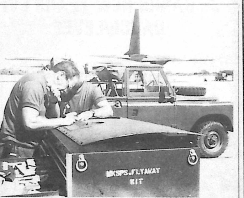
Sgt Claude Tremblay, left, and Master Cpl Denis Lavole (both of CFB Edmonton) repair a fastener on a Hercules aircraft panel. (Photo by Capt Renee MacTaggart.)
