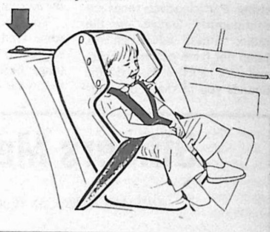
The tether strap must always be securely attached to a bolt installed in the rear shelf of a car, or on the floor of a van, station wagon or hatchback. Some automobile manufacturers provide pre-installed anchorage locations.
