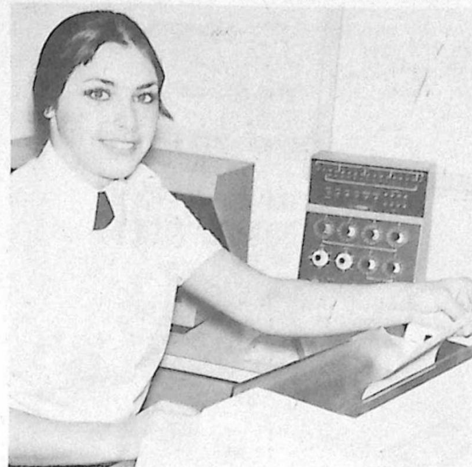
PRIVATE JOHANNE BROWN , 18 of Shawinigan, Que., a supply technician at National Defence Headquarters, Ottawa, operates a new computer terminal introduced into the Canadian Forces Supply System. A central computer automatically keeps records of stock inventory throughout the forces and resupplies bases when stock levels reach predetermined levels. The system was developed under the DEVIL program, an acronym for development of integrated logistics.
