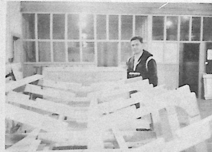
LAC B INGS hopes for a smooth fast ride from his "Sea Sled" inverted Vee speedster. This hull will go about 30 mph with a 25 horsepower outboard. Cost probably won't be more than $300 with full equipment including windshield and remote steering.
