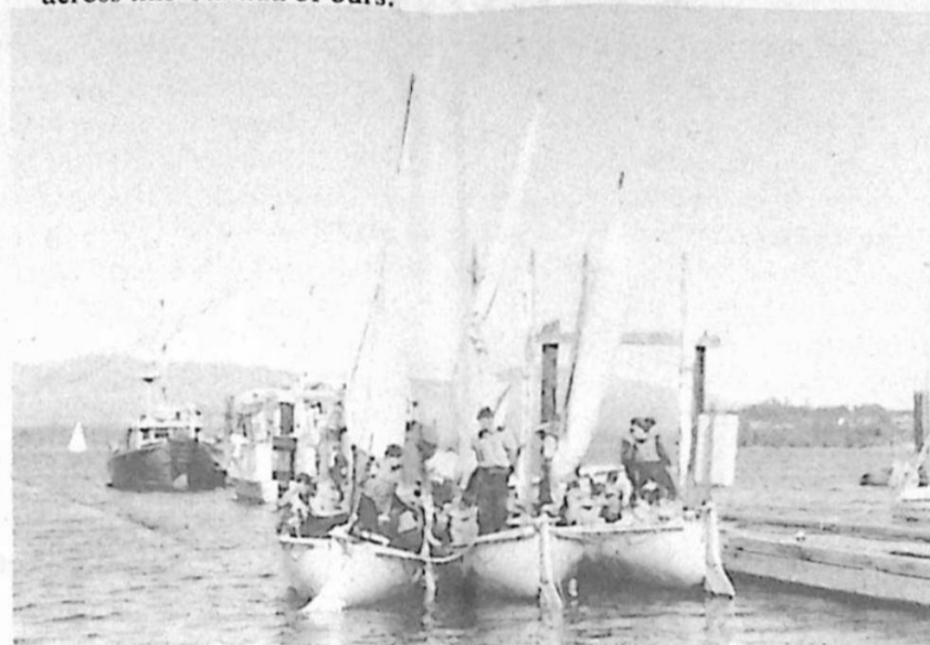
A whaler expedition prepares to slip for their 2 1/2 day sail. The 27' sailing/pulling whalers are equipped with radios and are known for their sea keeping capabilities. There are ten whalers at QUADRA. Whalers are carried aboard Her Majesty's Canadian Destroyer Escorts (DDE) and Helicopter Destroyers (DDH). Whaler sailing at QUADRA is where ADVENTURE BEGINS.
